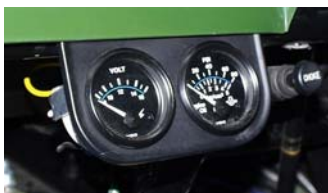
Oil, water & Volt Gauges
