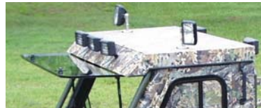
Visor mounted Lightbars feature 3 to 5 Halogens lamps. Unity Spotlights Rotate 360 dg. Requires battery and possibly alternator upgrade.
