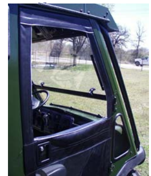
Lightweight Fabric covered doors fit all cabs. They feature a large zippered top window
