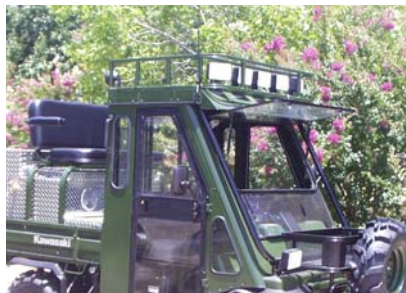
Visor and roof mounted Lightbars feature 3 to 5 spot and trapezoid Halogens lamps. Requires battery and possibly alternator upgrade.
