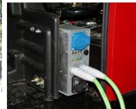
Bosch alternator, 25 amps of 110 volt power and 120 amp DC welder [Gas Models]
