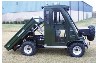
Electric bedlift. Economical, fast and strong lift screw.
